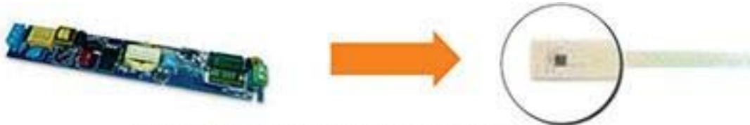
The driver was replaced by IC chip
