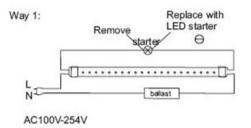
Turn off the power, remove fluorescent tube remove fluorescent starter and replace with LED starter. Place LED tube into position.
